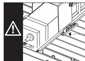
**!** Bubble level feature to precisely align luminaire with horizontal plane
