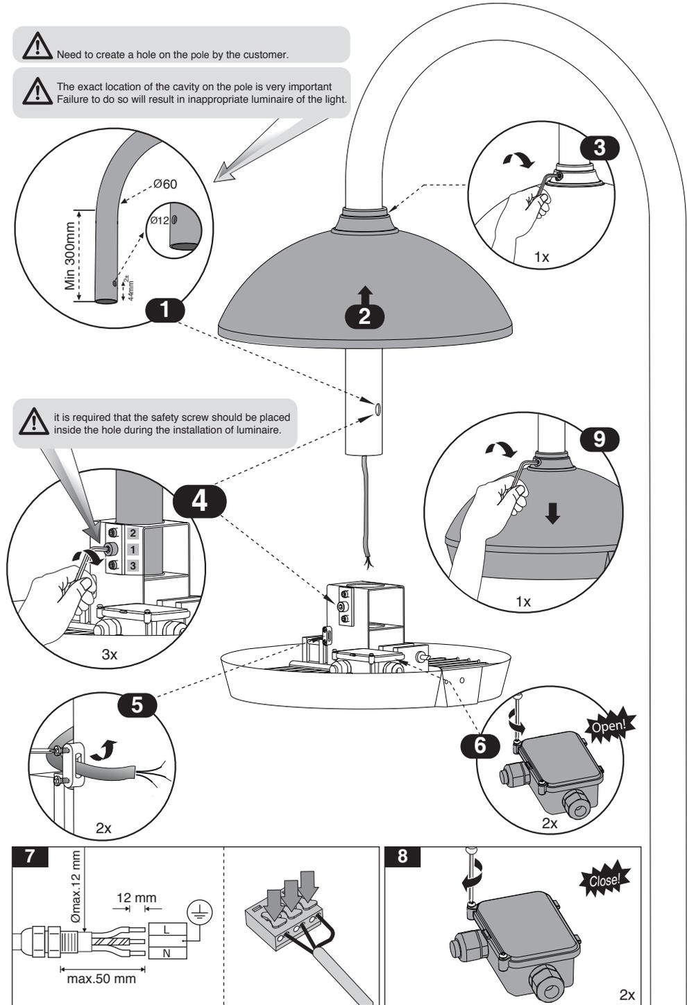
**EN SATURN** mounting horizontally to the pole instruction for installation and utilization
