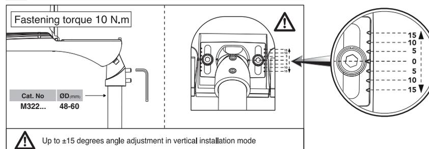
⚠ Up to ±15 degrees angle adjustment in vertical installation mode
