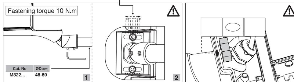
⚠ Up to ±15 degrees angle adjustment in horizontal installation mode, Bubble level feature to precisely align luminaire with horizontal plane
