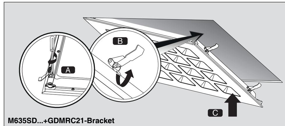
Installation accessories are used for integrated ceiling
