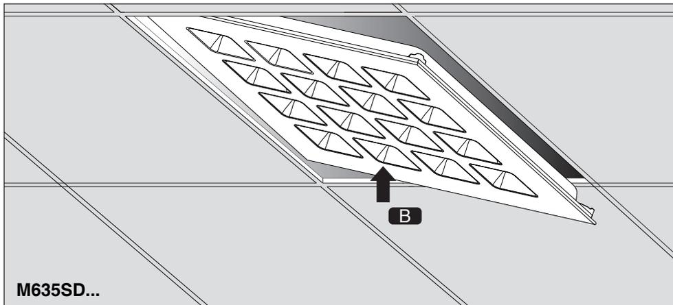
Mounting the LED panel in gypsum false ceiling
