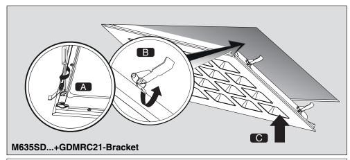
Installation accessories are used for integrated ceiling
